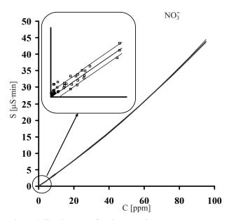
Fig. 2. Calibration curve for nitrate (V) ions.
