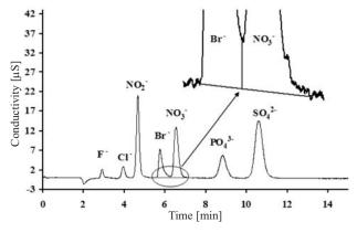
Fig. 3. Example of difficulty with correct integration of the peaks.
