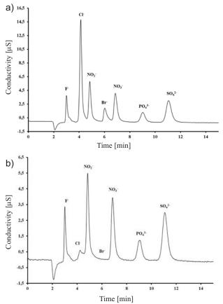
Fig. 1. The example of a chromatogram of investigated water before (a) and after (b) SPE purification.
